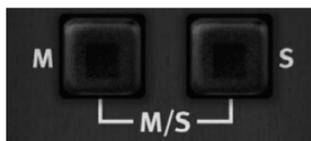
M/S encoding is only used for processing; decoding into L/R format is done before the signal is output. Note that both encoding and decoding is lossless.
