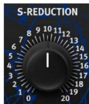
Scale values for the filter are displayed in dB. The actual reduction values, i.e. after phase cancellation, are shown in the S-Reduction display.
