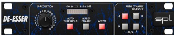
Back in the 1990's, we developed an alternative way to process signals in order to reduce sibilance based on phase cancellation. Unlike traditional compression methods, this procedure is much more unobtrusive and simplifies control to one single parameter. SPL's De-Esser quickly became a standard reference among recording studios, broadcast stations and live sound engineers.
